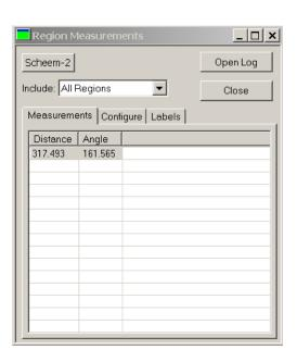
From (1) we can see that to get the correct angle ( $\alpha$ ) for the velocity calculation we need to subtract 90° from the one that MetaMorph gave us:
