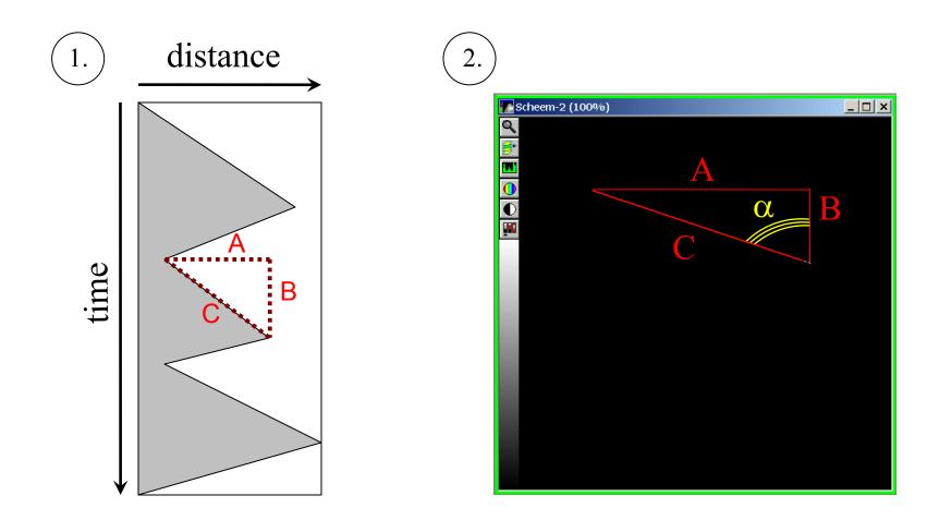
In the cartoon kymo drawn in (1), the line C represents a growth phase. If we make a right angled triangle as shown, then C is the hypotenuse. We can make an angle between C and B... lets call it  $\alpha$ , see (2).
