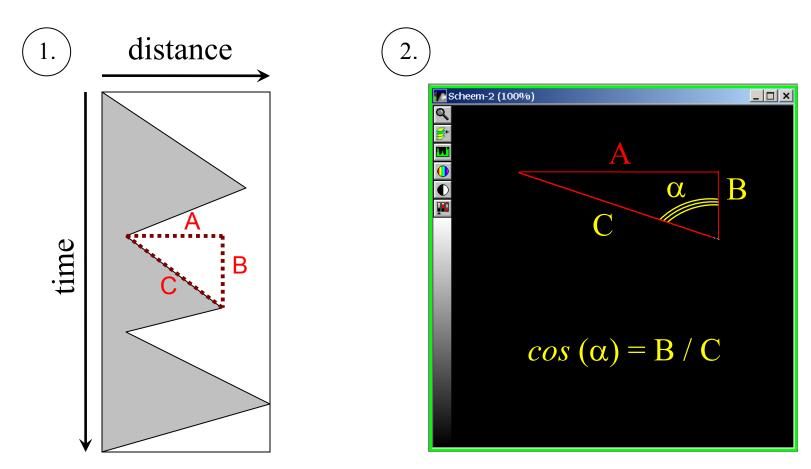
We can do the same thing for duration/time. In this case time would equal the length of line B multiplied by a factor dependent upon angle  $\alpha$ . Note, that in (1) time is explicitly defined in the vertical axis at 90°.
