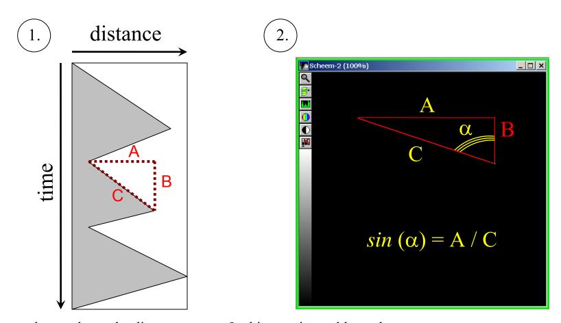
We can also work out the distance grown. In this case it would equal the length of line C multiplied by a factor dependent upon angle  $\alpha$ . Note, that in (1) distance is explicitly defined in the horizontal axis at 90°.
